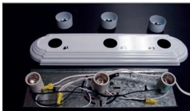
**Fig. 2.** The lighting fixture is simple to take apart and rewire.
